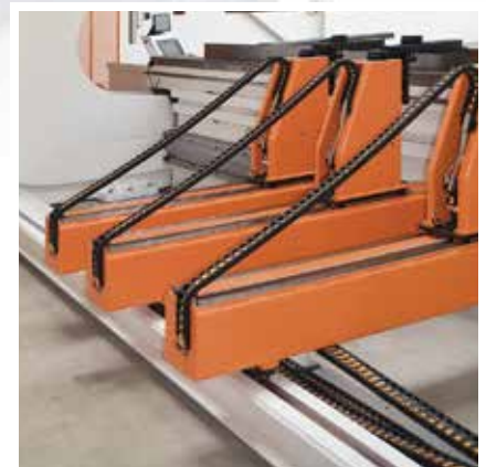
9 axis independent tower type backgauge.
